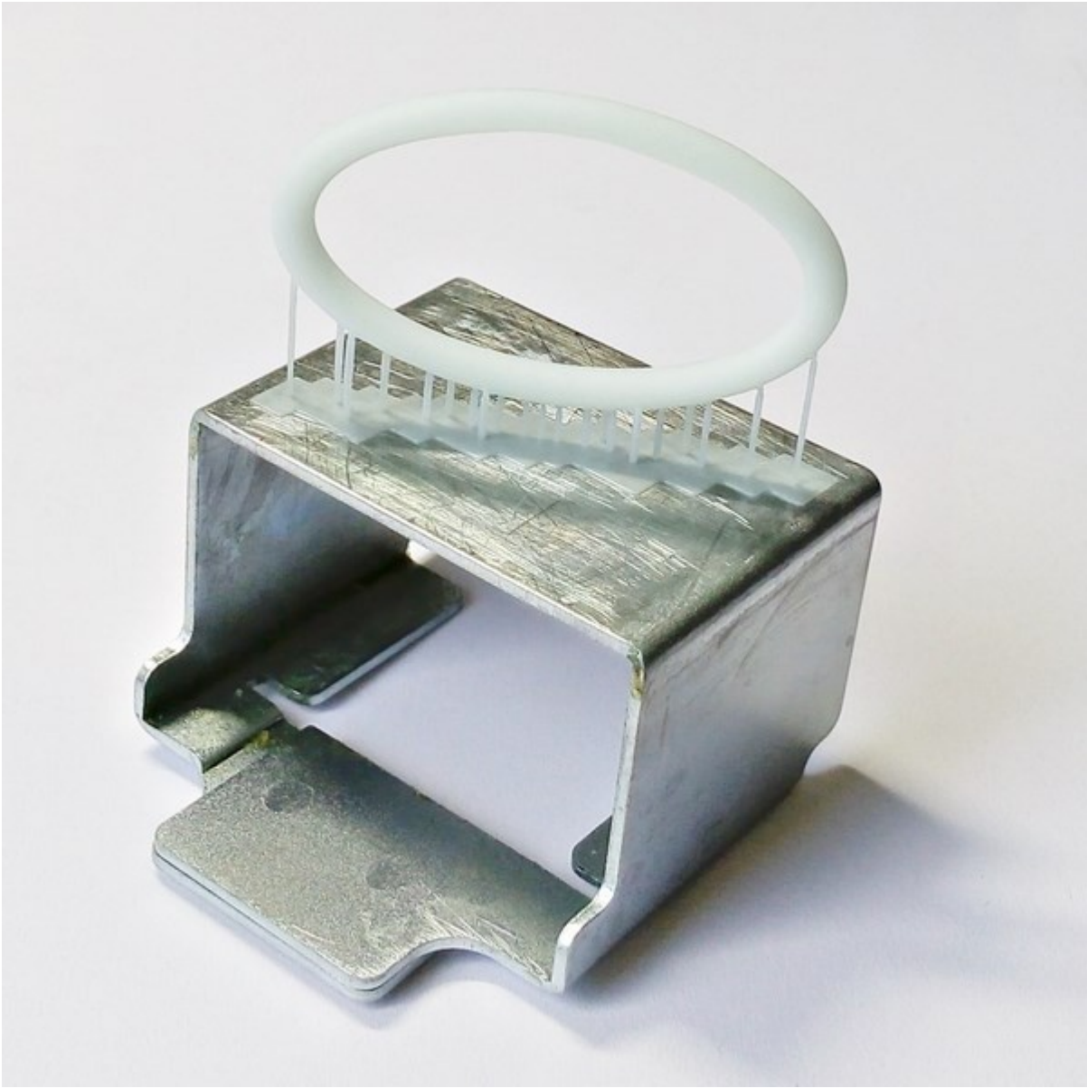
Perfect print of snow white resin on the 1200 projet, with thin supports
