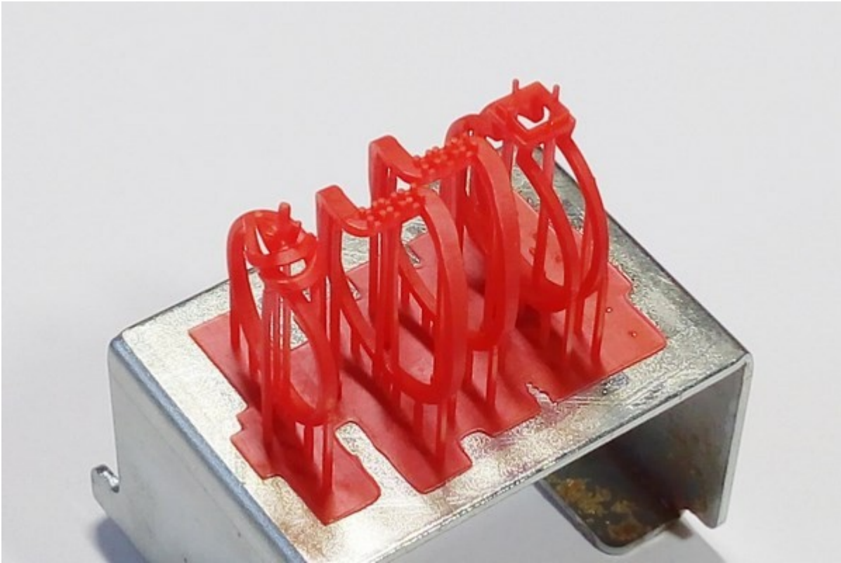
Rings printed with castable FTD resin on the 1200 projet
